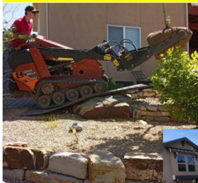
Mini Skids (left) require a minimum of 43" access. 48" for trees 10' and taller or 4" caliper & bigger.
